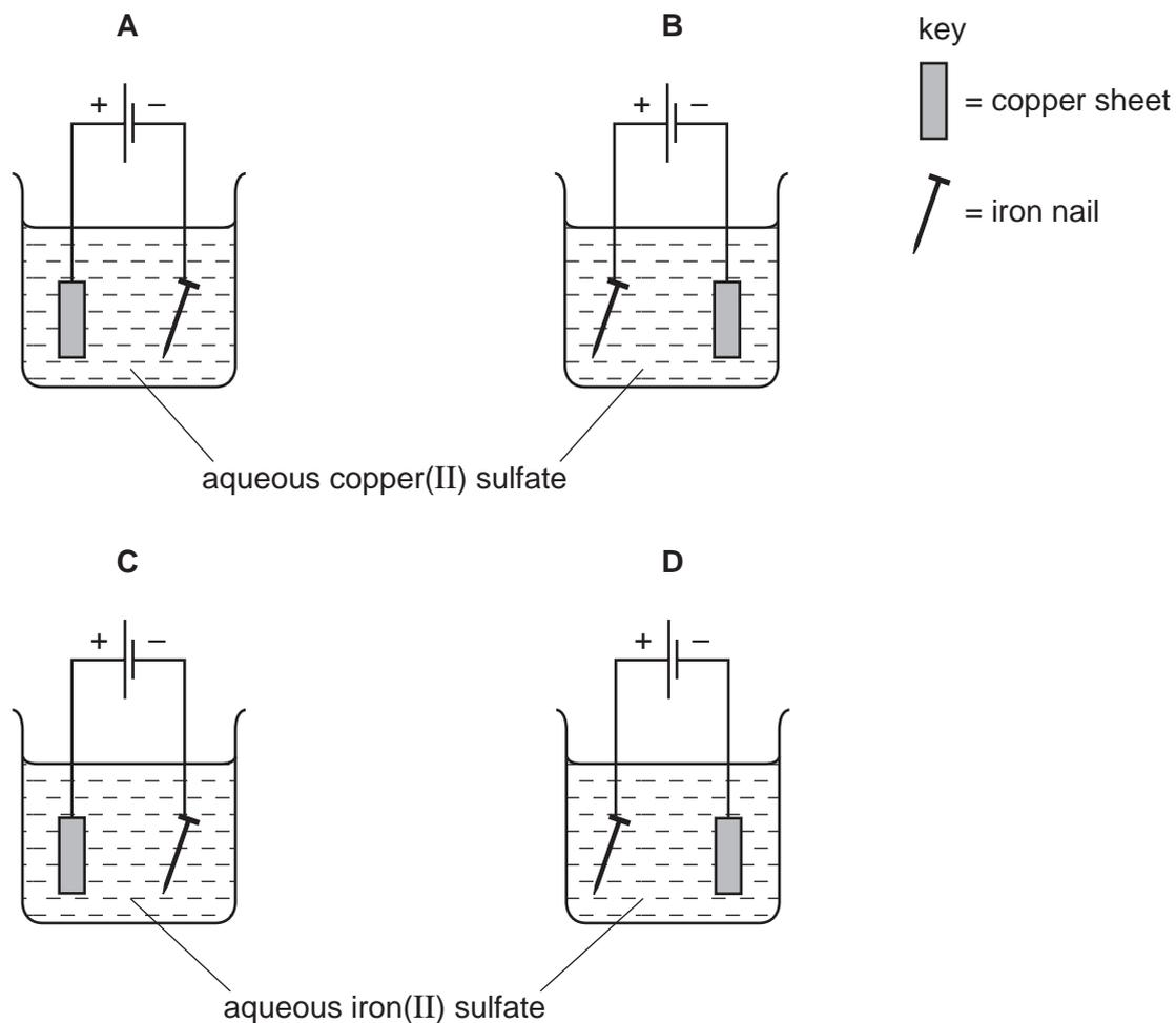
11 The diagram shows two different metal strips dipped into an electrolyte.
