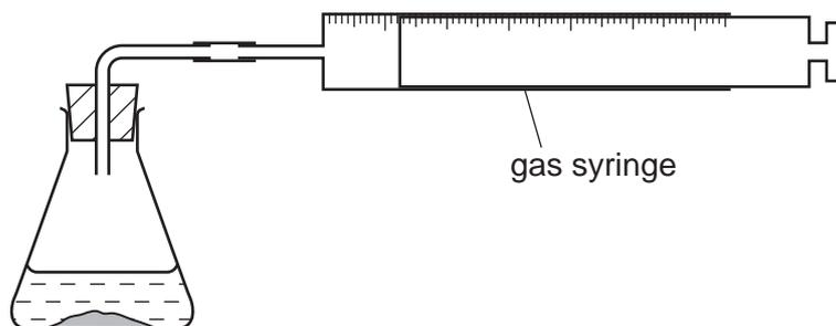
The volume of gas given off is measured at different times and the results plotted on a graph.
